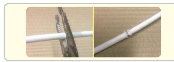
Step 2 - Twist the polymer coating to break the bond with the wire
